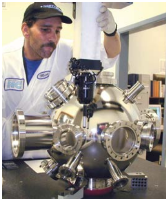
Mechanical inspection of process chamber with CMM (coordinate measuring machine)
