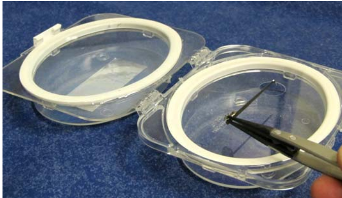
Figure 3-22: Lifting the Stylus from Its Case
