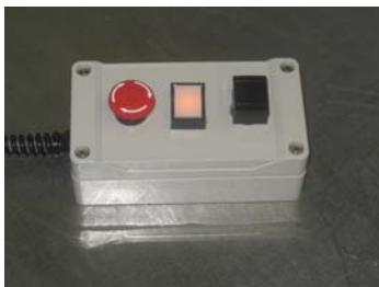
Figure 3-3: EMO Box with Illuminated On Button
