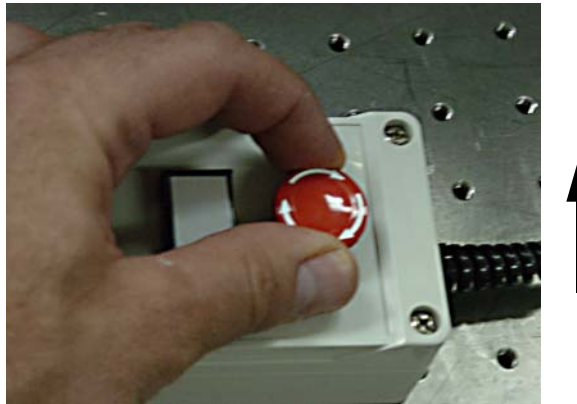
Figure 3-2: Releasing the Red Emergency Off Button on the EMO box
