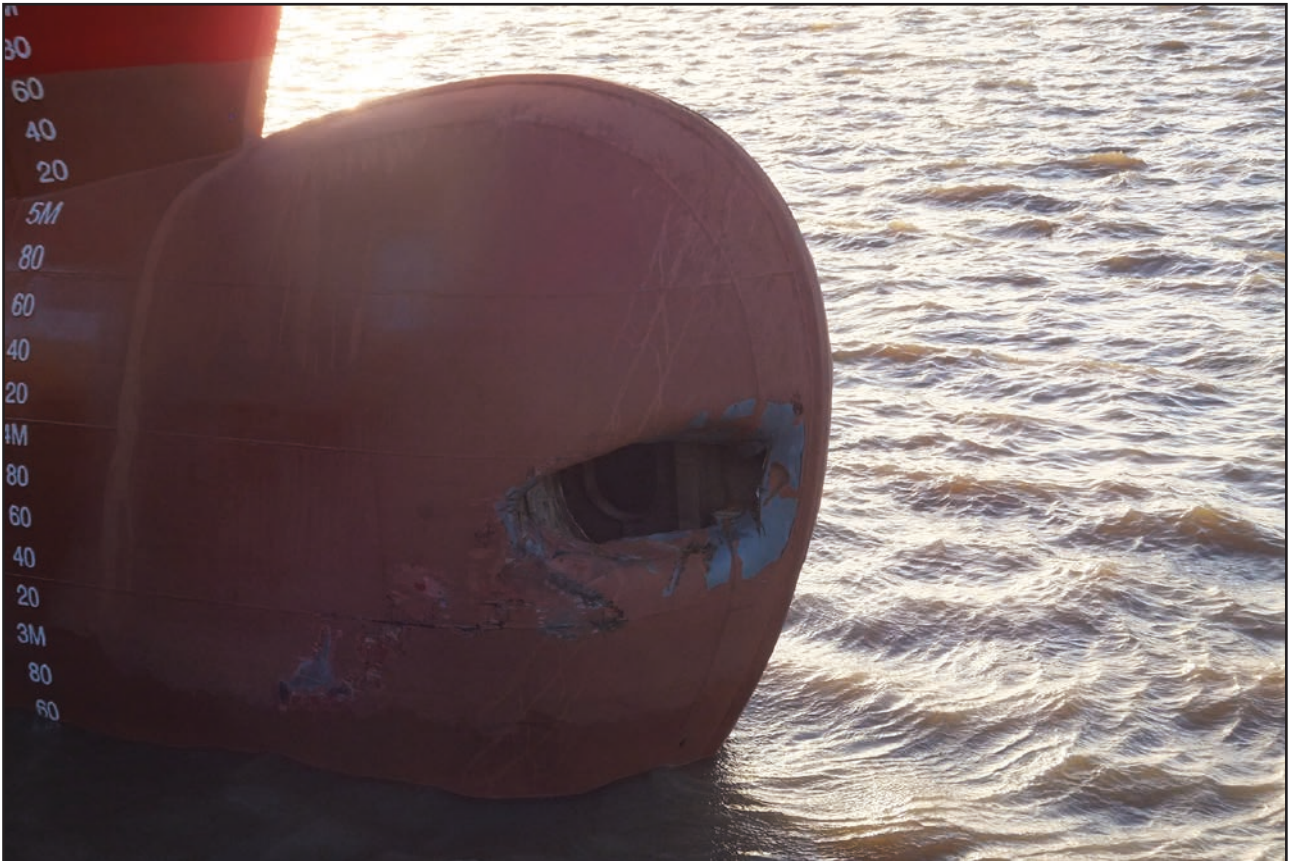
Figure 1: Bulbous bow damage caused by contact with the quay
