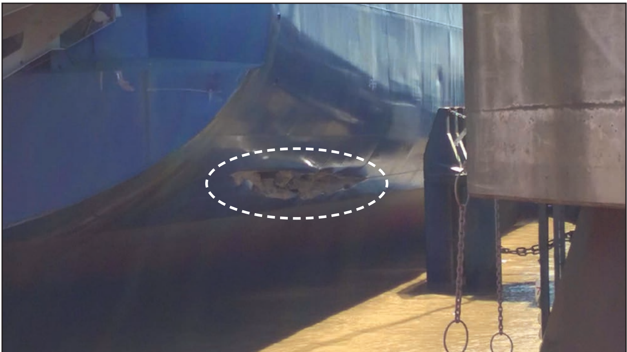
Figure 1: Damage sustained to the vessel
