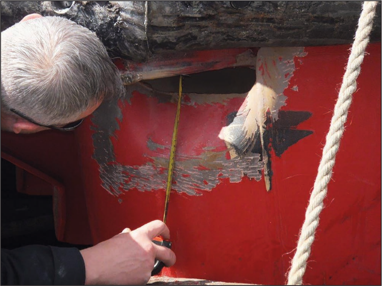
Figure 1: Vessel was holed above waterline
