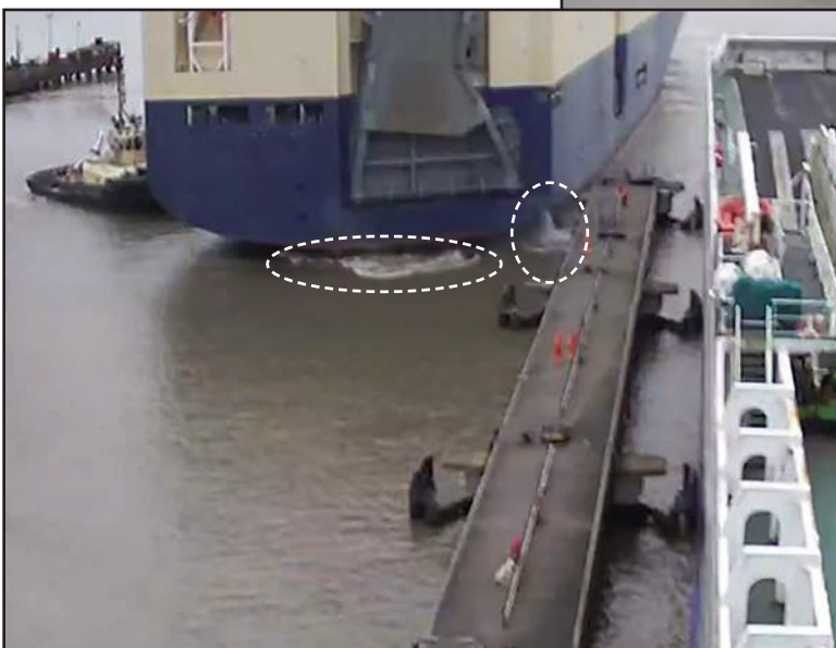
Figure 4: Vessel engine and rudder used after collision and damage to tank causing leak
