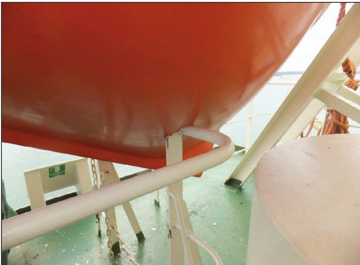
Figure 2: Lifeboat hull damage
