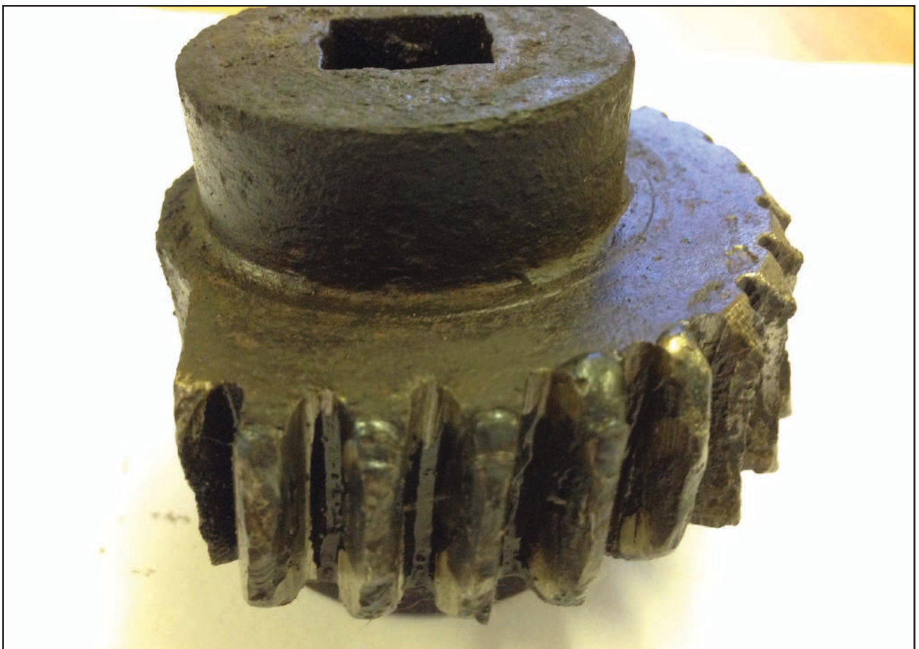
Figure 3: Gearbox quadrant, showing signs of damage and previous repair
