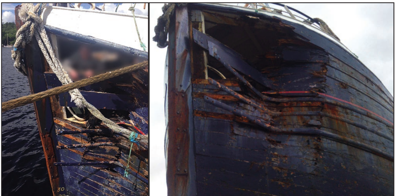
Figures 1 and 2: Damage to vessel A's port bow area
