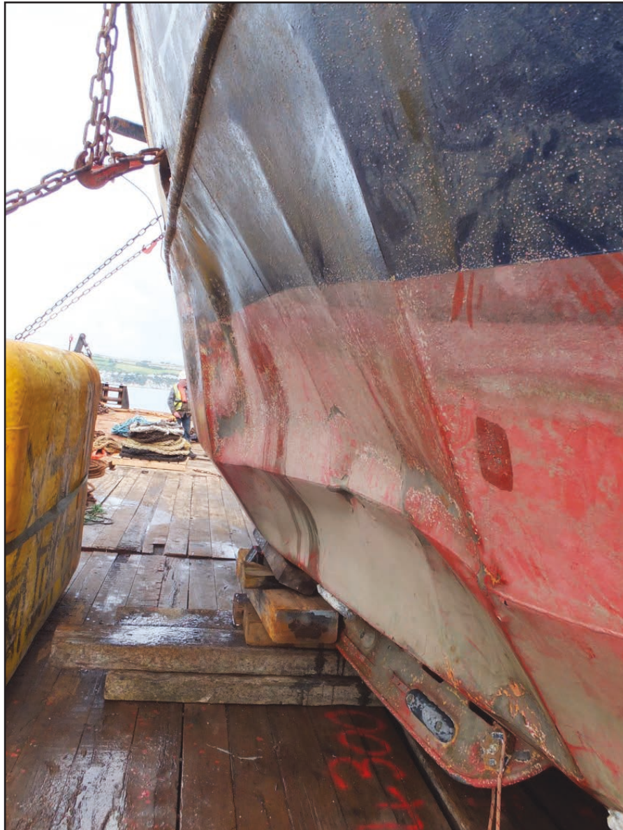
Figure 26: Implosion damage to JMT 's starboard side
