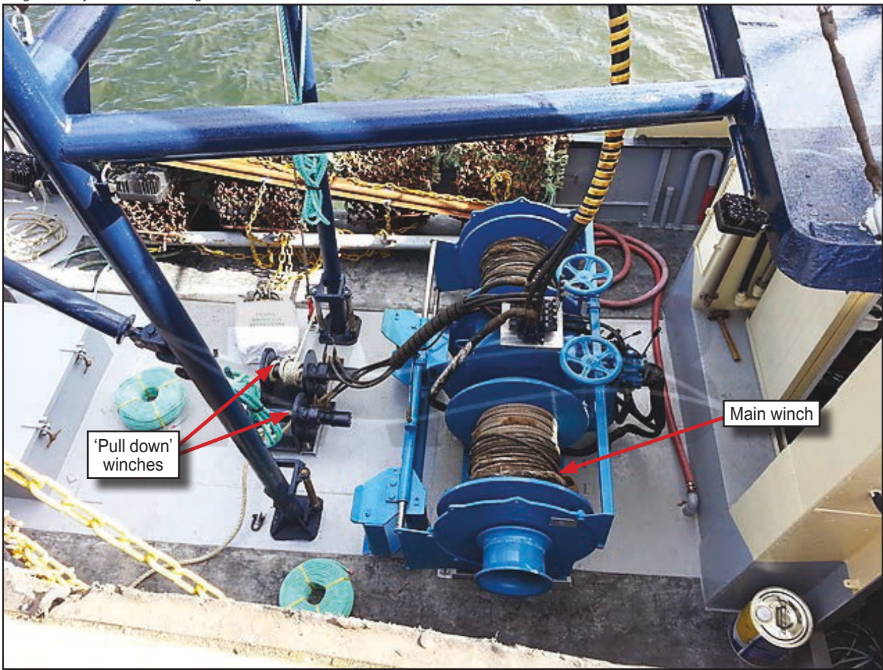
Figure 2: JMT 's working deck
