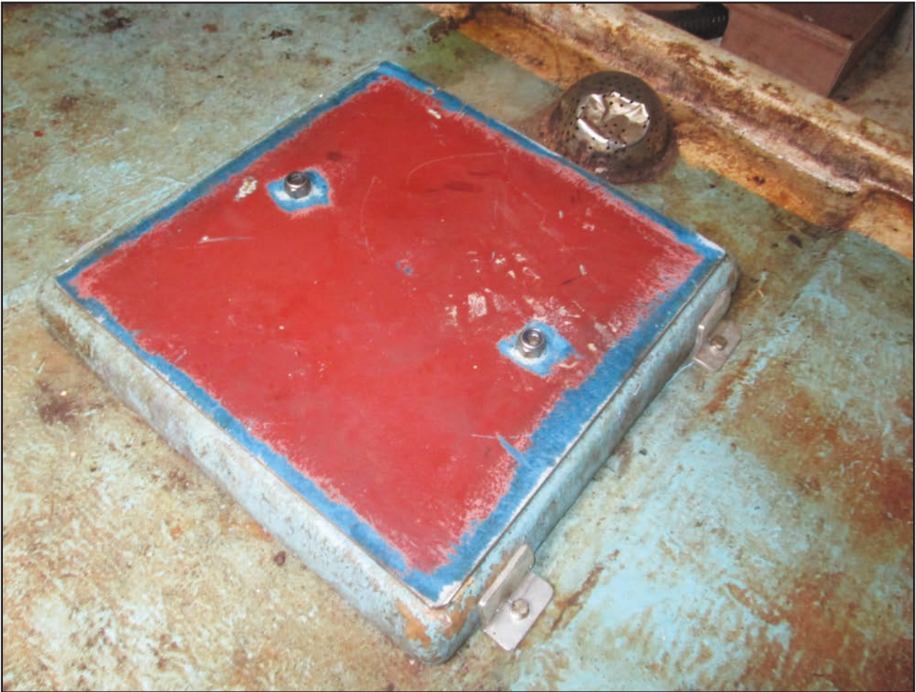
Figure 9: Shaft inspection hatch in JMT 's fish hold floor
