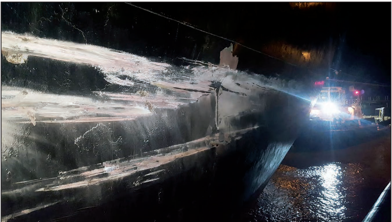
Figure 1: Damage to ship's port side
