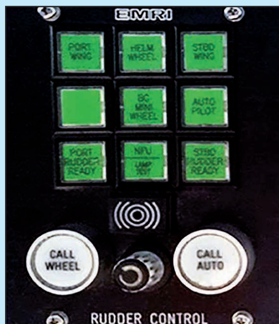
Figure 2: Helm control station indicator light panel
