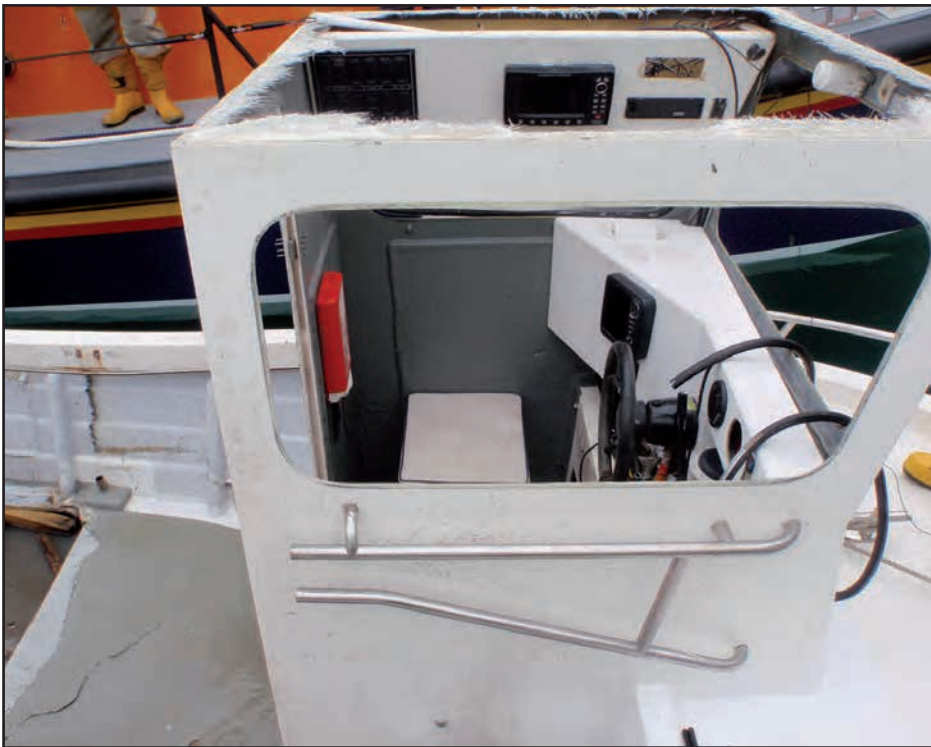
Figure 1: Wheelhouse with missing roof and windows
