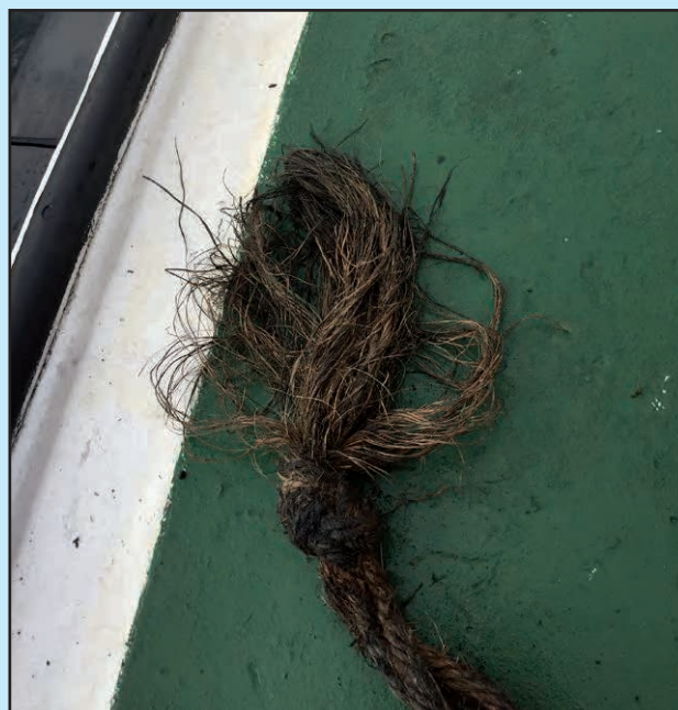
Figure 3: Ladder side rope showing contamination
