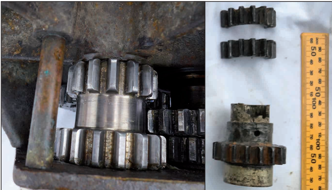
Figure 2: Port and starboard side winch pinions
