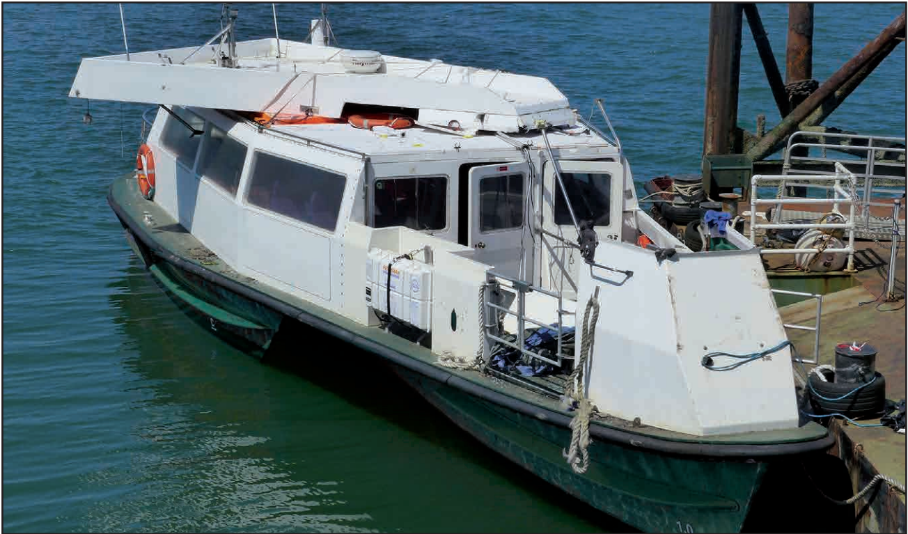
Figure 2: Ferry post-collision showing the demolished wheelhouse
