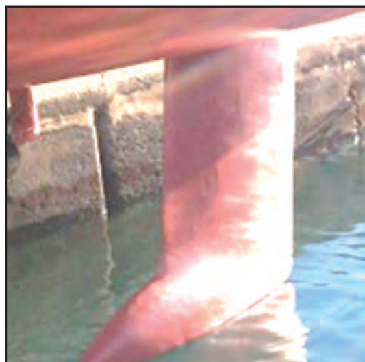
Figure 2b: Shallow draught, lead keel, fitted to Tyger of London , subject of this safety bulletin
