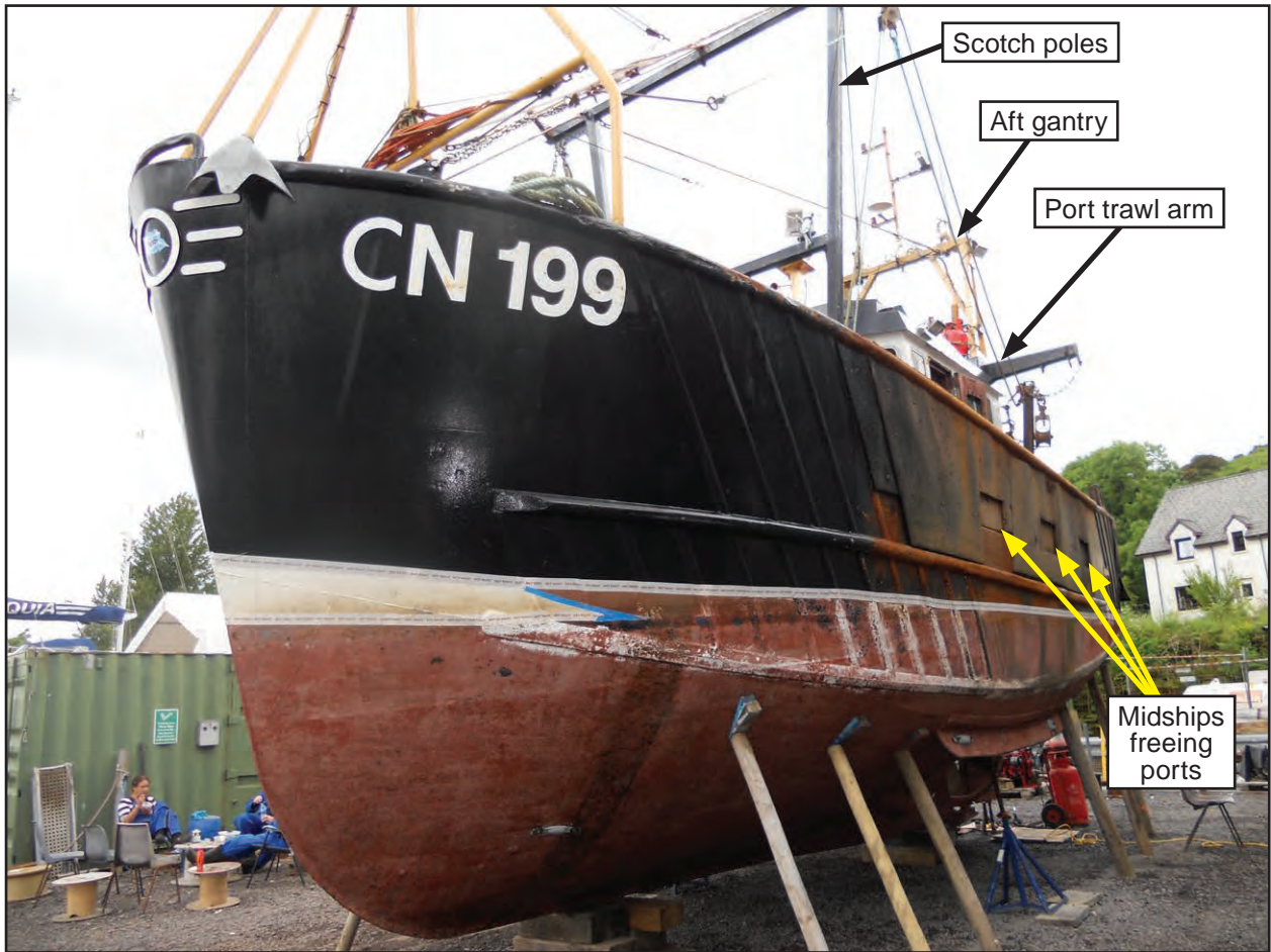
Figure 11: Pre-purchase survey – hull form forward port side
