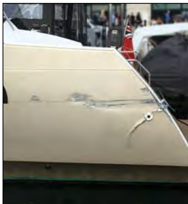
Figure 2: Collision damage to the catamaran's port quarter
