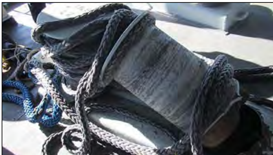
Figure 1: Mooring bitts' failure during tug operation
