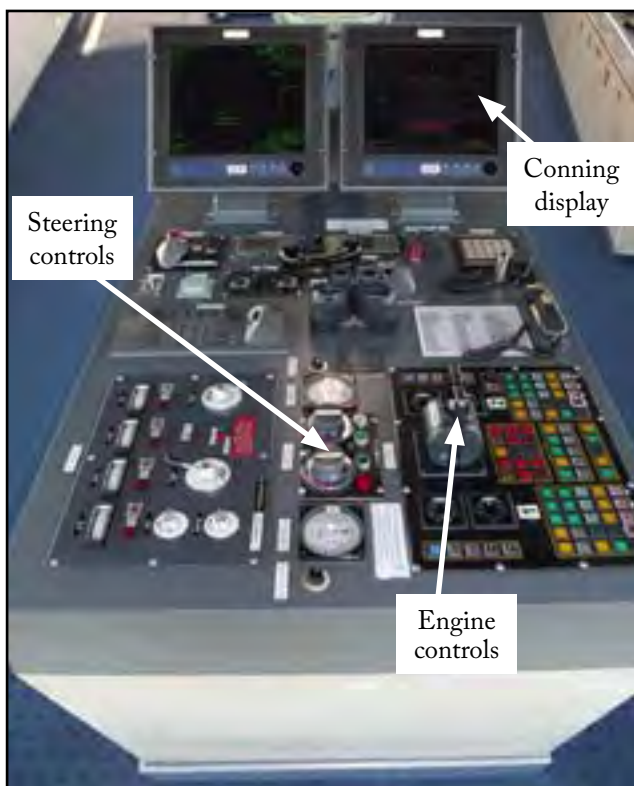
Figure 1: Port bridge wing console
