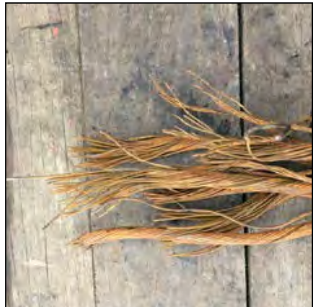
Figure 1: The broken towing wire
