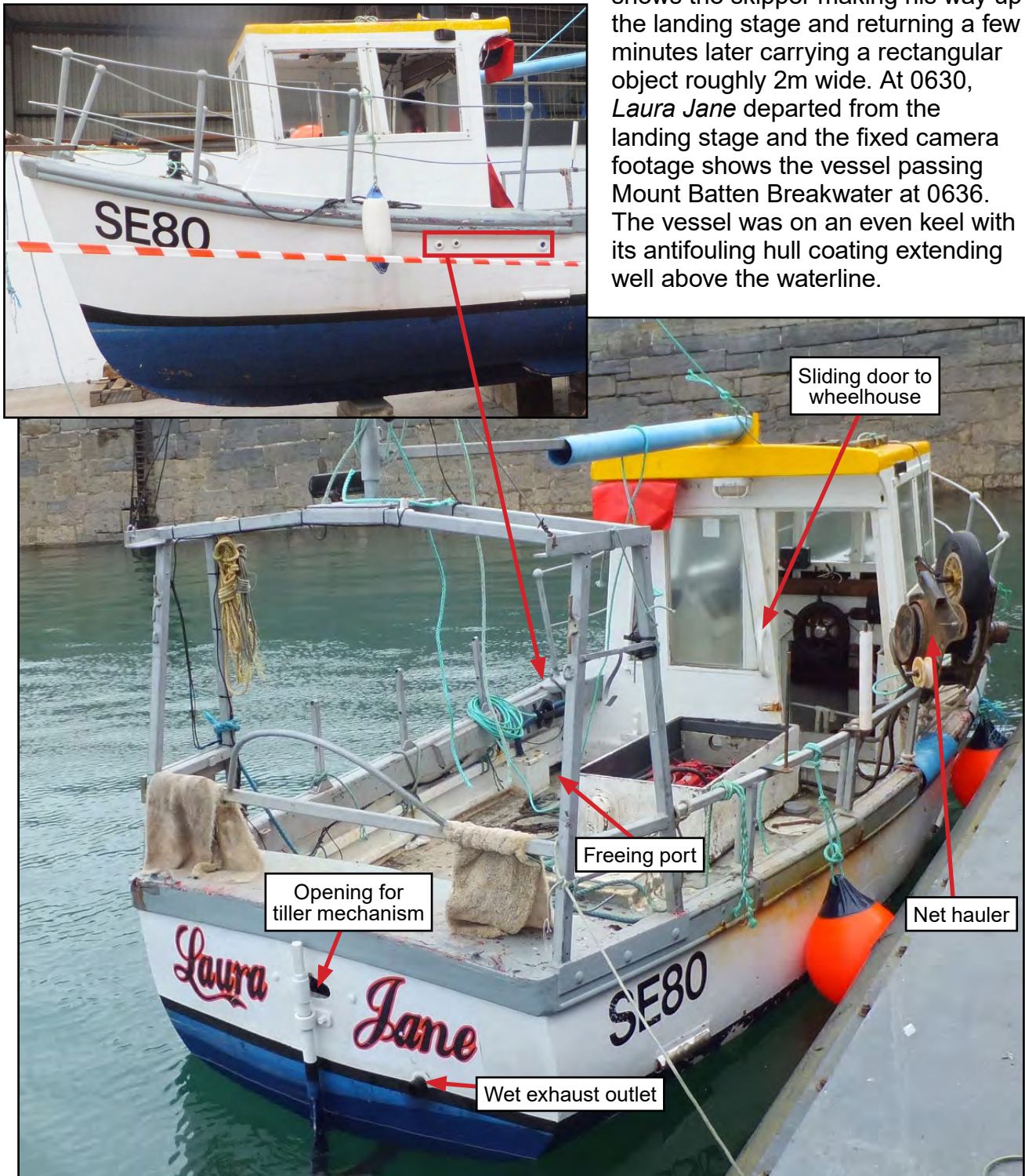
Figure 1: Laura Jane (inset: bilge overboard discharges)
