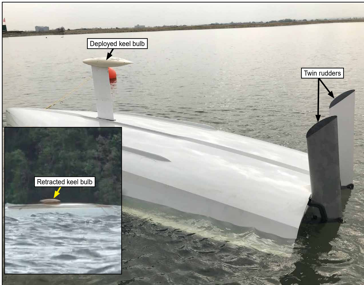
Figure 2: Inverted boat with a fully deployed keel bulb (Inset: the keel bulb hard up against the inverted hull)
