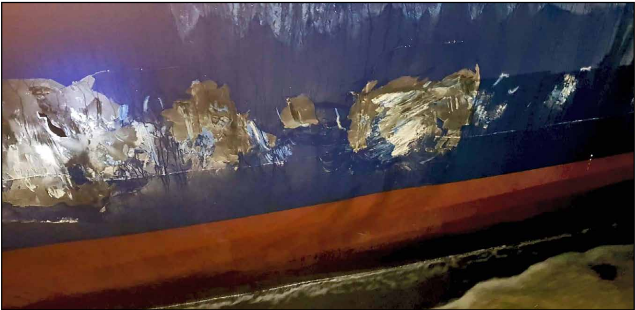
Figure 2: Detail of hull damage to the ferry's port side after impact with the adjacent quay wall
