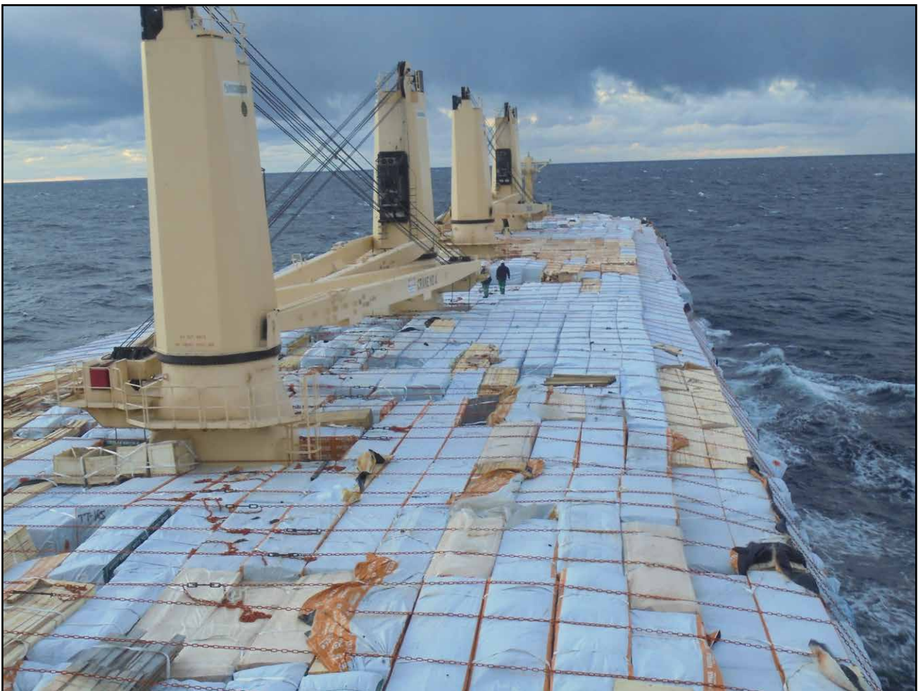
Figure 1: Timber deck cargo secured with top-over lashings at sea
