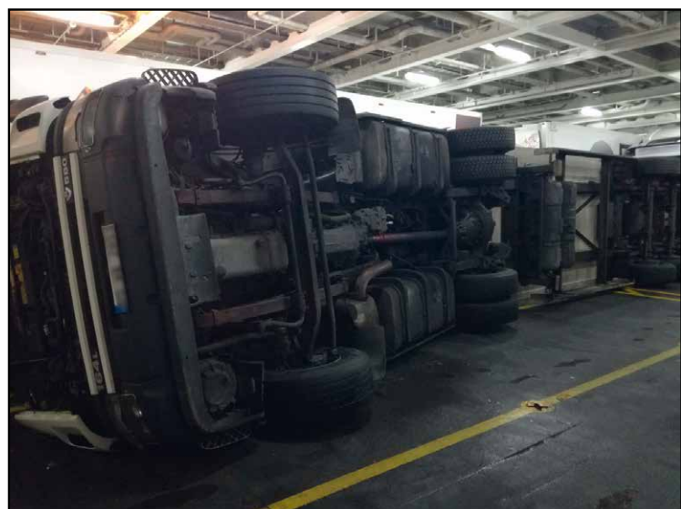
Figure 3: Truck toppled over on main deck
