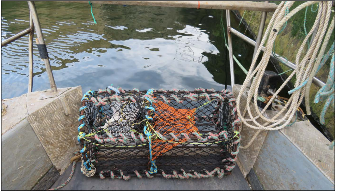
Figure 7: Creel jammed in shooting gate
