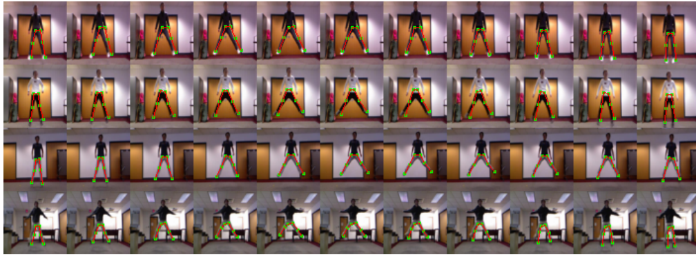
Figure 3: Pose estimation using the proposed semi-supervised adversarial constraint learning approach. r_\theta takes in single image and outputs the 2-D location of 6 joints (in green). Lines (in red) are added automatically. The images show results across 4 test groups (horizontal strips) when only 3 out of 28 training groups were directly labeled.
