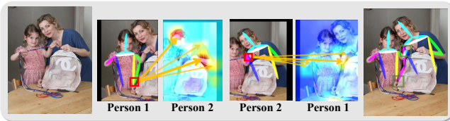
Figure 5: Inter-Human Attention Visualization. The incorrect region (marked in the red box) is corrected with the aid of higher response regions, which are indicated by the orange arrows.
