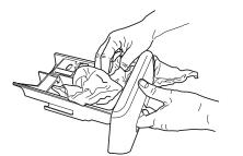
**5.** Reinstall the detergent dispenser and push it back into the detergent compartment.
