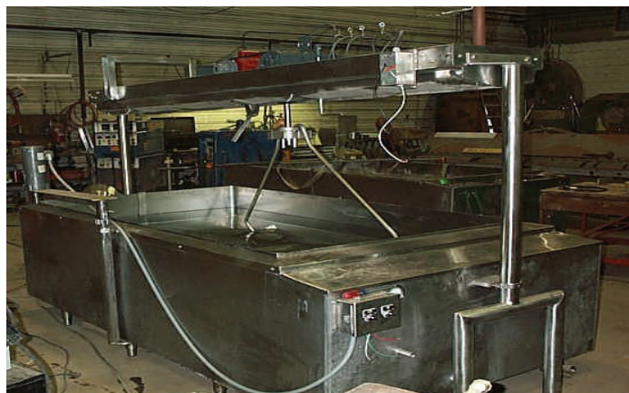
PHOTO OF 500 GALLON DUO-VAT W/ NEW SANI-STIR TRAVELING AGITATOR
