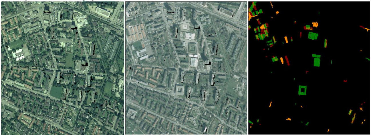
Figure 3. The experiment result. Left: orthophoto in the year 2002; middle: orthophoto in the year 2007; right: change detection results (red: demolished; green: new building; orange: uncertain changes).
