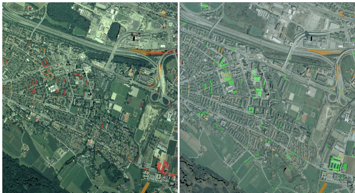
Figure 4. The result of a large area: Left: orthophoto in the year 2002; middle: orthophoto in the year 2007; (red: demolished; green: new building; orange: uncertain changes).
