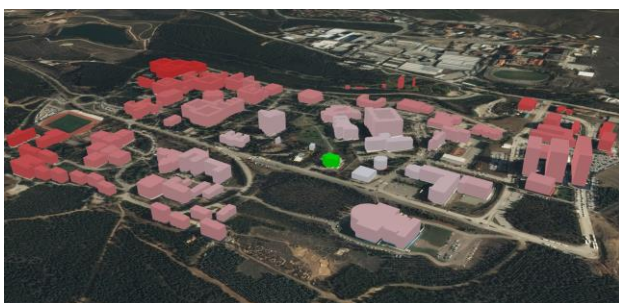
Figure 6. Buildings colored by distance to a landmark (Geomatics Engineering Department building depicted with green) on Cesium.
