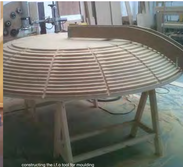
constructing the i.f.o tool for moulding
