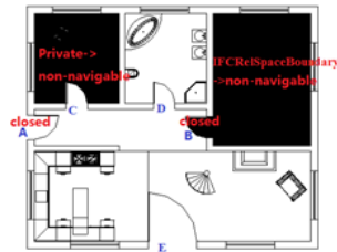
Figure 4. Single floor semantic information extraction in Building 1 (Unpassable area in black, passable area in white)
