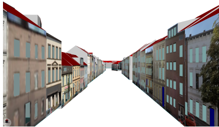
Figure 10. LoD3 building models with windows, doors and textures, visualized with FZKViewer.
