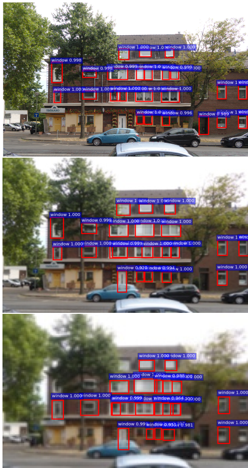
Figure 3. Example for problems in window detection on low resolution images. From top to bottom: original resolution ( 2590 \times 1715 pixel), 1/16 of the original resolution and 1/32 of the original resolution.
