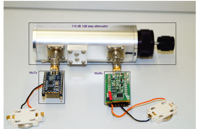
Figure 16. Assembled WuRx PCB and attached to a host node.
