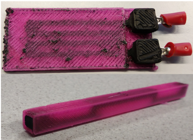
Figure 14. 3-D printed integrated strain sensors.
