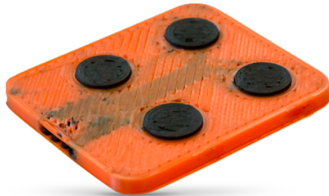
Figure 17. Photograph of 3-D printed sEMG electrodes, printed using a combination of conductive and dielectric TPU (Wolterink et al., 2017).
