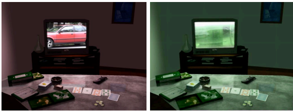
Figure 2: A streaming video texture used on the screen of a TV set. The video content is also used for dynamic lighting of the room.
