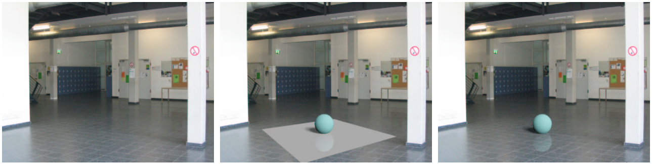
Figure 8: An in-shader differential rendering example. A sphere is rendered into a video background (left) using the AR view compositing method from [PMWS03, PS04]. Stand-in geometry (mid) is used to render the visual cues. The differential rendering method allows to blend the effects with the real background (right).
