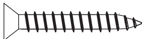
#12 x 1 1/2" Phillips Flat Head Sheet Metal Screw Use 9/64" Drill bit Also: #12 x 1"
