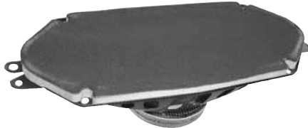
DVC-1001 Speaker 4" x 10" Dual Voice Coil Speaker • 120 Watts Peak Power • 4 Ohm Impedance • Sensitivity 87dB 46 Hz • 19KHz • 12 oz. Magnet
