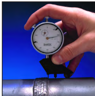
MEASURES UNDERCUT BUTT WELD
