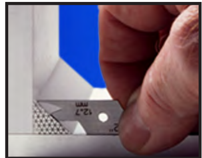
CHECKING THROAT DIMENSION
