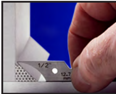
CHECKING WELD LEG SIZE
