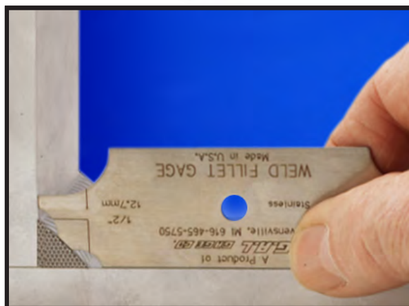
CHECKING FILLET THROAT SIZE
