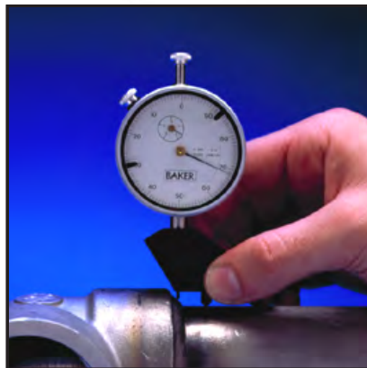
MEASURES UNDERCUT SOCKET WELD
