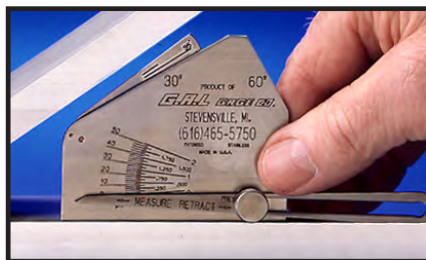
CHECKING ANGLE OF VERTICAL MEMBER
