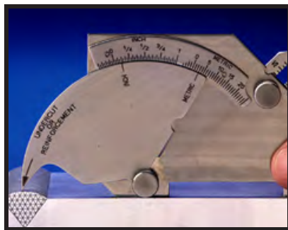
Excess Weld Metal
