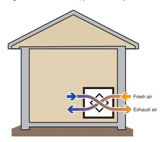
Balanced system - whether an ERV or a HRV, the concept is the same for a balanced whole house system. Incoming fresh air is filtered and tempered with outgoing exhaust air. Location of the device is usually dependent on the AHU blower and ductwork for the house.
