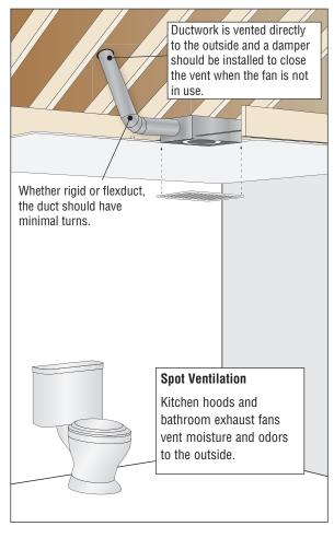
should include dampers that close when the fans are not in use. Always select ENERGY STAR labeled fans to ensure quiet and efficient performance.
