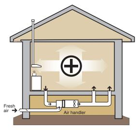
Fresh air intake vent - a small outside air duct connected to the return creates desirable positive pressure and can be controlled to operate regularly. If the house pressure is slightly positive compared to outdoors, pollutants such as pollen will not be pulled inside.
