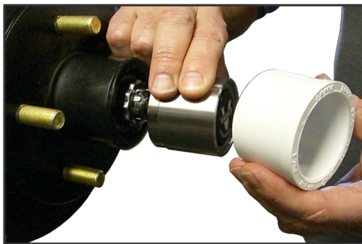
Place PVC collar over protector (2"x1-1/2" slip collar for 1980 size) (2" female adapter for 2328 size) in order to prevent damage to the protector during installation.
