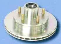
Heavy duty ventilated rotors dissipate heat rapidly by allowing cooling between the inner and outer brake surfaces. Rotor surface temperatures can rise rapidly from repeated stopping or slowing on mountain grades. Only ventilated rotors can stop this heat from building up to unacceptable levels. Less expensive, non-ventilated rotors overheat causing rapid brake pad deterioration, excessive rotor surface wear and rotor warping.
