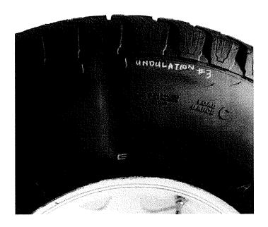
The condition, sometimes referred to as sidewall undulations, is a common characteristic of radial tire construction (see photo). These indentations are more noticeable in larger/wider radial-ply tire sizes and become more visible with higher inflation pressures.
