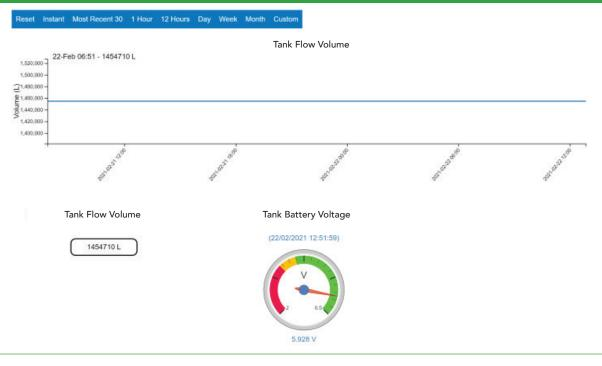
Using cellular or radio connection, a range of different size flow meters can be monitored and recorded. Current flow, flow rate and cumulated flow can be calculated and displayed.
