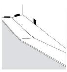
Attach the second plank of the new row by aligning the short side tongue of the second plank with the groove of the first plank while keeping the long side edge about a quarter inch away from the first row. Continue laying remaining panels in this manner.
