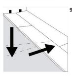
Angle the two pieces up by about 20 degrees and then as the second-row plank into position tight to the first-row plank, using a tapping block if needed. Tap the plank three times, first where the two planks meet, second across from the joint in the previous row and third at the far side of the plank
