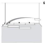
Begin the next row with the off-cut piece from the previous row to stagger the pattern. Pieces should be a minimum of 8" (20 cm) long and joint offset in adjoining rows should be at least 16 (40 cm).
