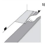
Continue connecting the first row until you reach the last full plank. Fit the last plank by rotating the panel 180° with the pattern side upward, place beside row, mark and then saw off excess. Attach as described above.
