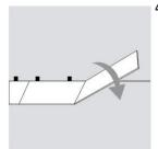
4) To attach your second plank, insert the short edge tongue of the second plank into the short edge groove of the first plank holding the second plank at an angle. Lock the short ends together by lowering the second plank into place. The planks should be flat to the floor.
