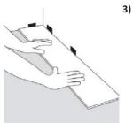
Start in a corner by placing the first plank with its trimmed side facing the wall. Use spacers along each wall to maintain an expansion space of 3/8" (10 mm) between the wall and the flooring.
