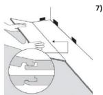
To start your second row, tilt and push the side tongue of the plank into the side groove of the very first plank at about 30°. Press the second plank down flat and the tongue will
