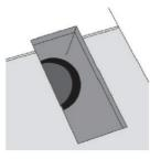
11) Door frames and heating vents also require expansion room. First cut the plank to the correct length. Then place the cut panel next to its actual position and use a ruler to measure the areas to be cut out and mark them. Cut out the marked points allowing the necessary expansion distance on each side.
