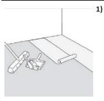
For planks without pre-attached cushion, install foam underlay. Run the foam underlay in the same direction as the flooring panels. Underlay should be butted side by side with no overlap. Tape seams together. Do not install an additional underlayment under planks with pre-attached cushion.
