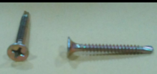
C/SK Posi Head Self drill / tap Screws. 4x22mm BZP finish.
