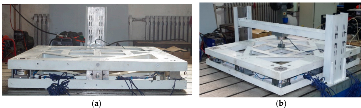
Figure 10. Calibration experiment setup for force loading of the proposed six-dimensional sensor in (a) the X-direction and (b) the Z-direction.
