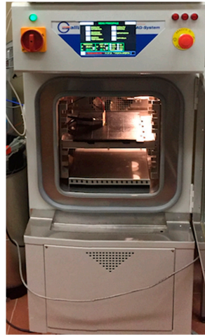
Figure 12. Picture of the setup used for the characterization of the temperature sensor.
