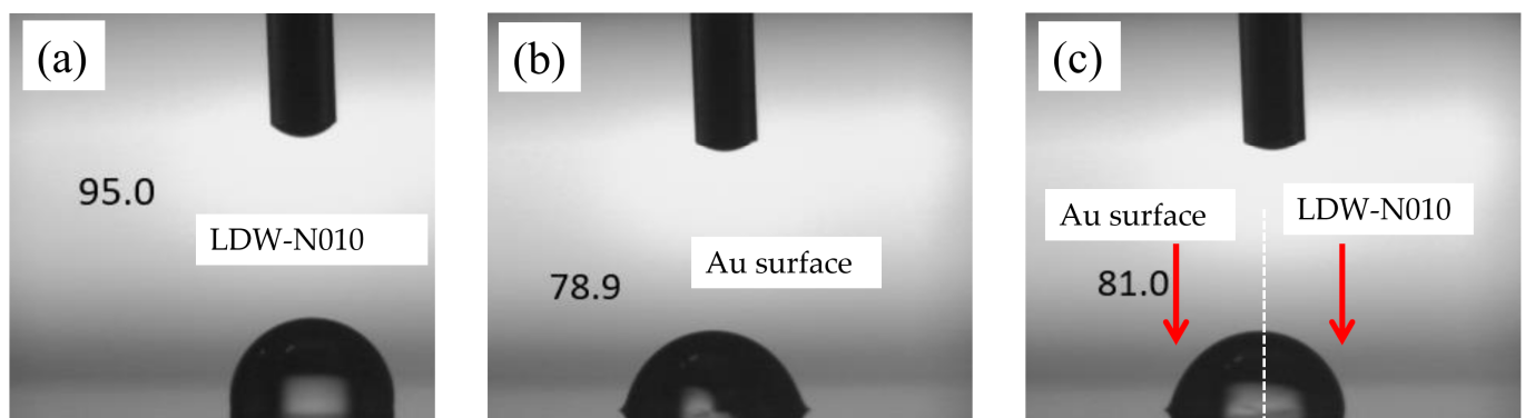
Figure 6. Measured contact angle on (a) LDW-N010 surface; (b) Au electrode surface without LDW-N010; (c) interface surface between Au and LDW-N010.
