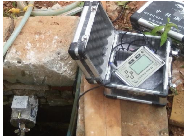
Figure 3. Installation diagram of blast vibration meter.
