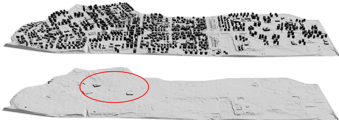
Figure 4. An overview of the generated digital surface model (DSM) and the digital terrain model (DTM), showing one area (red) with DTM filtering errors.
