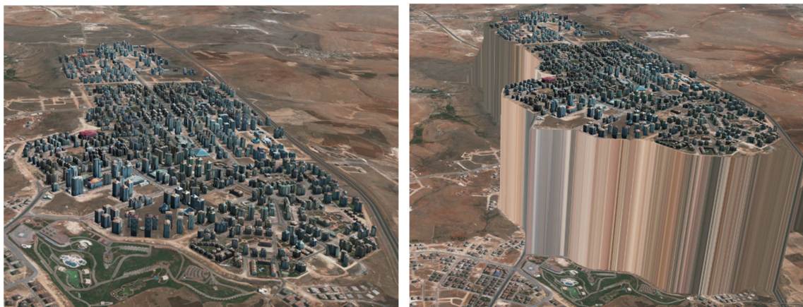
Figure 13. An example of Cesium World Terrain merged ( left ) and unmerged ( right ) with the high-resolution DTM and with the textured LoD2 model in the study area.
