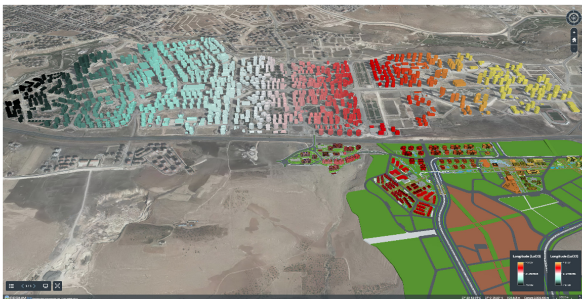
Figure 18. LoD2 building models model colored with their longitudes using 3D Tiles styling.
