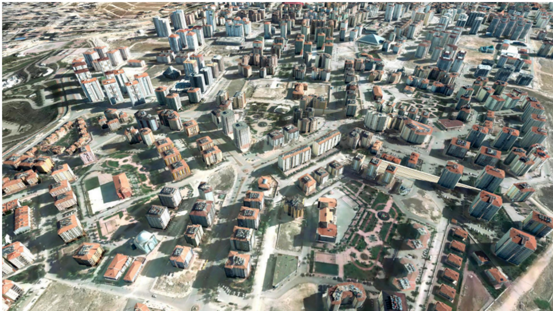
Figure 5. Unity Game Engine visualization of the textured LoD2 model together with the DTM and the true-orthophoto basemap.
