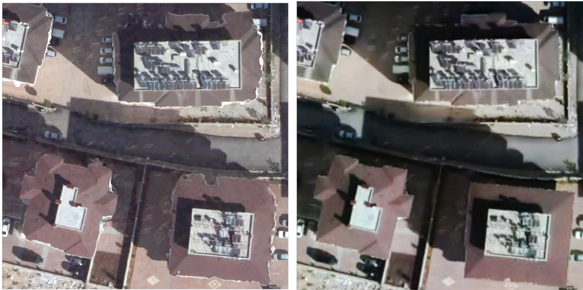
Figure 15. Radiometric comparison of ordinary orthophoto product (left) and the true orthophoto (right). The differences are especially noticeable at the roof edges.
