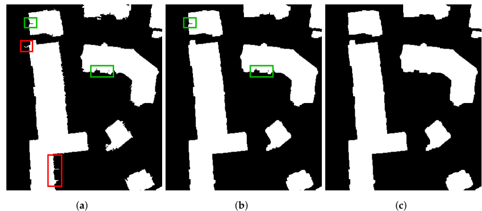
Figure 5. Illustration of postprocessing after the region matching of our building mask refinement method. (a): An enlarged building mask after our region matching method, which has the same spatial range as Figure 3a. (b): (a) after being processed by the second morphological opening operation. (c): (a) after being processed by both the second morphological opening and the second closing operation.
