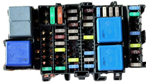
Figure 3. Real fuse box with fuses and relays.
