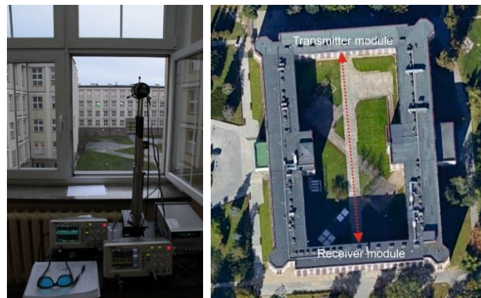
Figure 11. The laboratory stands for testing the FSO link outside the Military University of Technology building.
