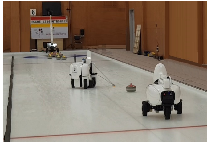
Figure 11. Experiment on creating a return path using the return path algorithm in an actual curling field.
