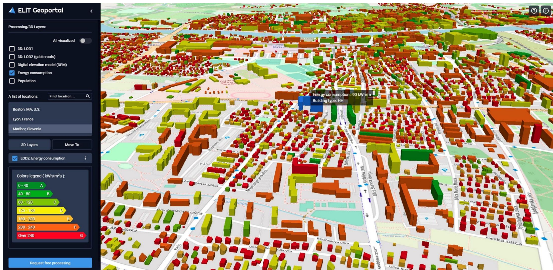
Figure 10. A fragment of a whole urban area of the city of Munster, Germany, presented on the Geoportal as 3D City GML LOD1 models with the implemented use case of estimation of energy consumption by buildings.
