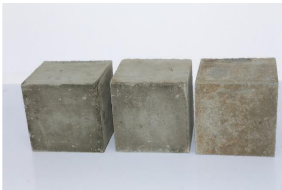
Figure 13. The appearance of aerated concrete obtained by a non-autoclave method with the same concentration of fullereneol-m (0.028 mass.% relative to cement).
