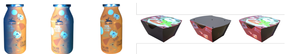
Figure 6. Results obtained for the mixed prototypes with a dual-projection setup according to the two types of blending techniques implemented: standard blending (left) and sharp edge (right).
