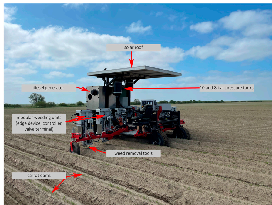
Figure 1. The multi-track weeding robot on a carrot field of our cooperation partner Westhof Bio GmbH in Friedrichsgabekoog, Germany.
