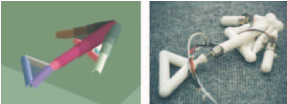
Figure 3.27: A crawling robot evolved by Lipson and Pollack [74]. The left panel shows the simulated robot, and the right panel shows the corresponding physical robot. Reproduced with kind permission of Dr. H. Lipson.
