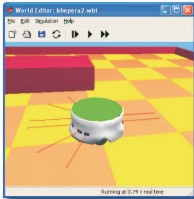
Figure 3.28: A screenshot from a Webots™ simulation of a Khepera II robot. Reproduced with kind permission of Dr. O. Michel, Cyberbotics.
