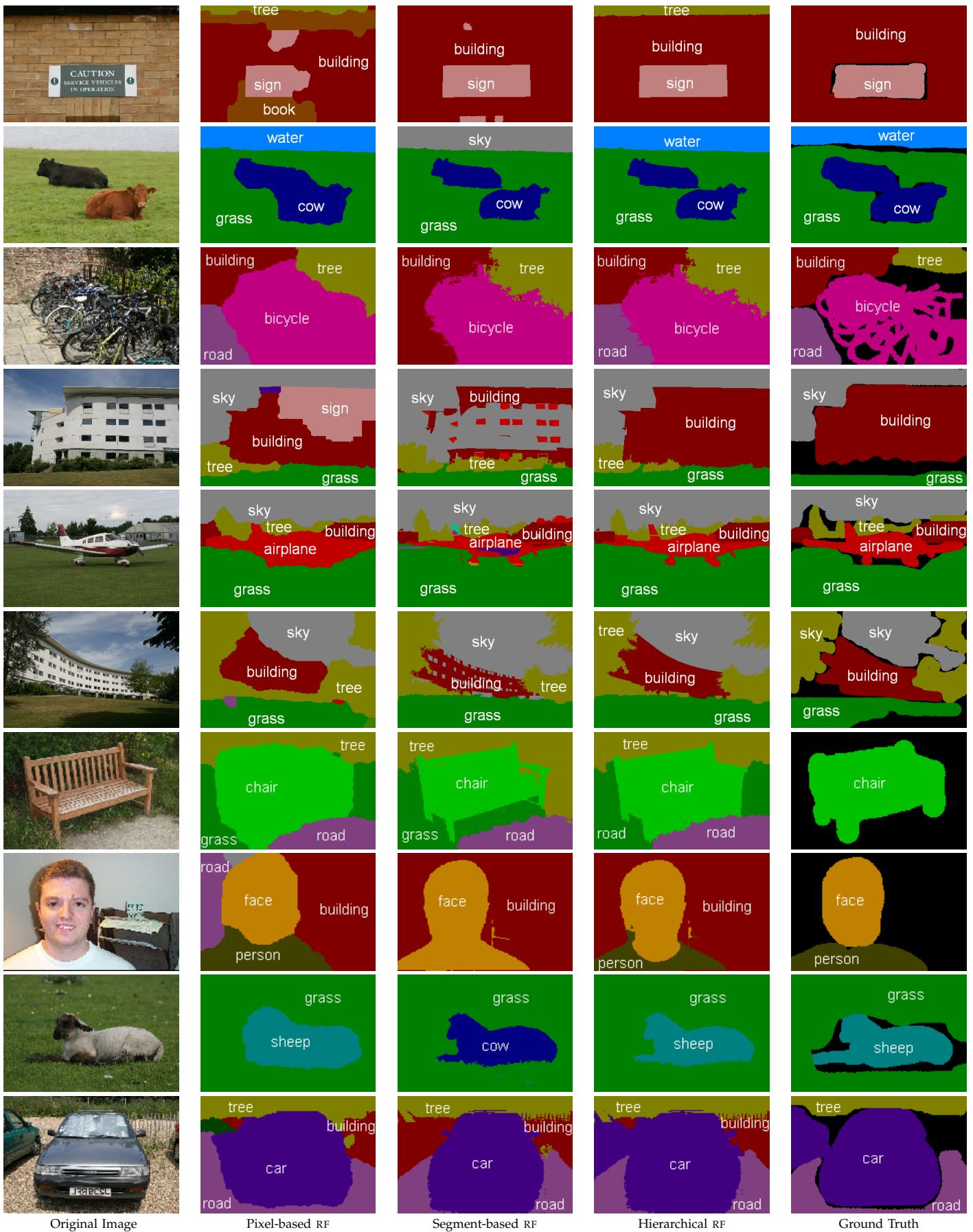
Fig. 6. Qualitative results on the MSRC-21 data set comparing non-hierarchical (i.e. pairwise models) approaches defined over pixels (similar to TextonBoost (Shotton et al, 2006)) or segments (similar to (Pantofaru et al, 2008; Russell et al, 2006; Yang et al, 2007) described in section 3) against our hierarchical model. Regions marked black in the hand-labelled ground truth image are unlabelled.
