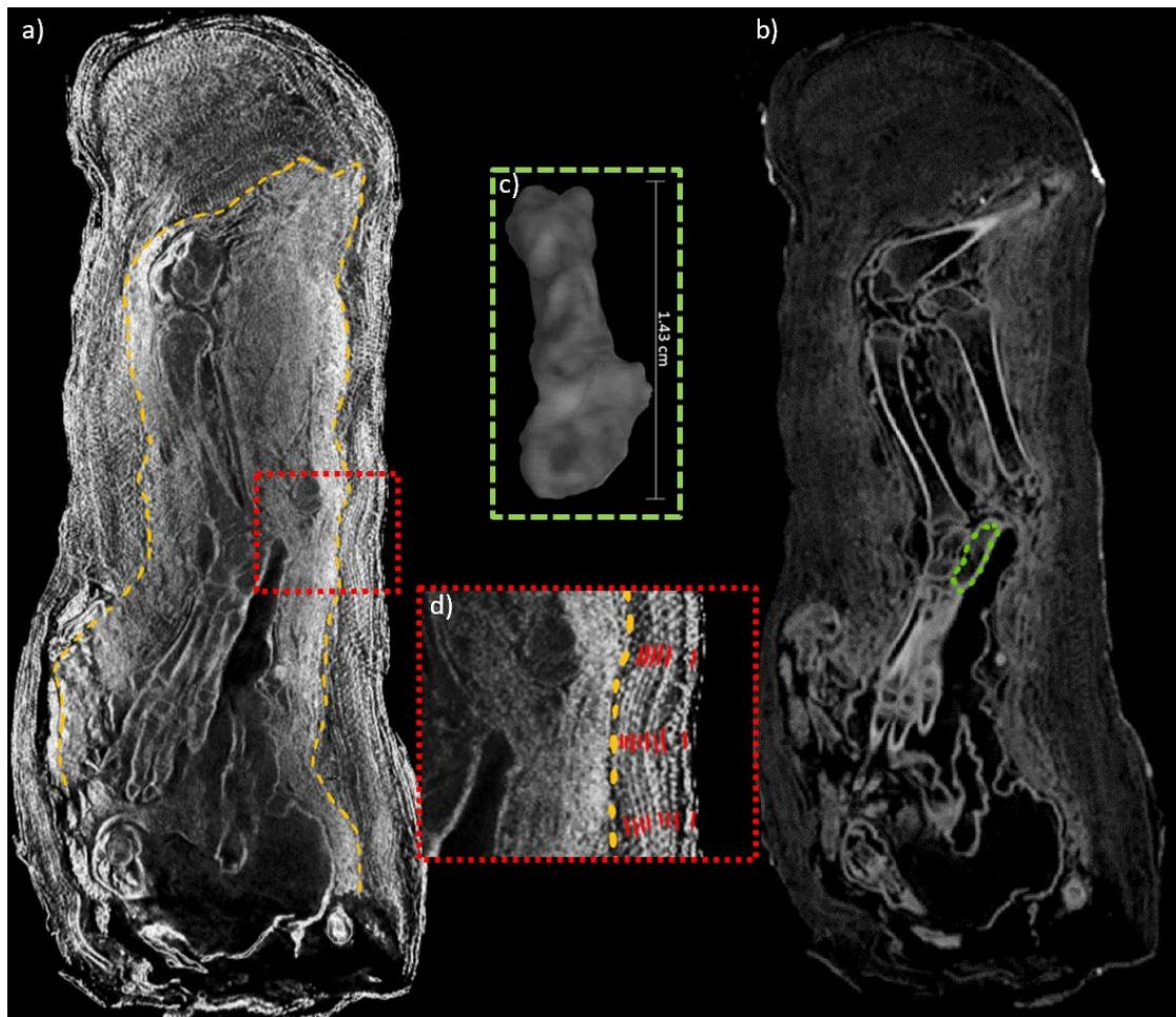
*Figure 5. a) Neutron CT slice shows layers of textile wrapping; b) X-ray CT slice shows higher grayscale contrast; c) Segmented and visualised calcaneus bone [green area in b)]; d) Close up showing layered wrapping of varying tightness and coarseness [red box on b)].*
