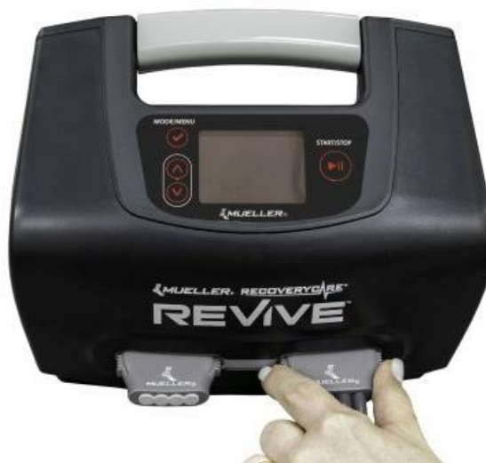
Figure 20 - Connecting the Garment Hose Bundle to the Console
