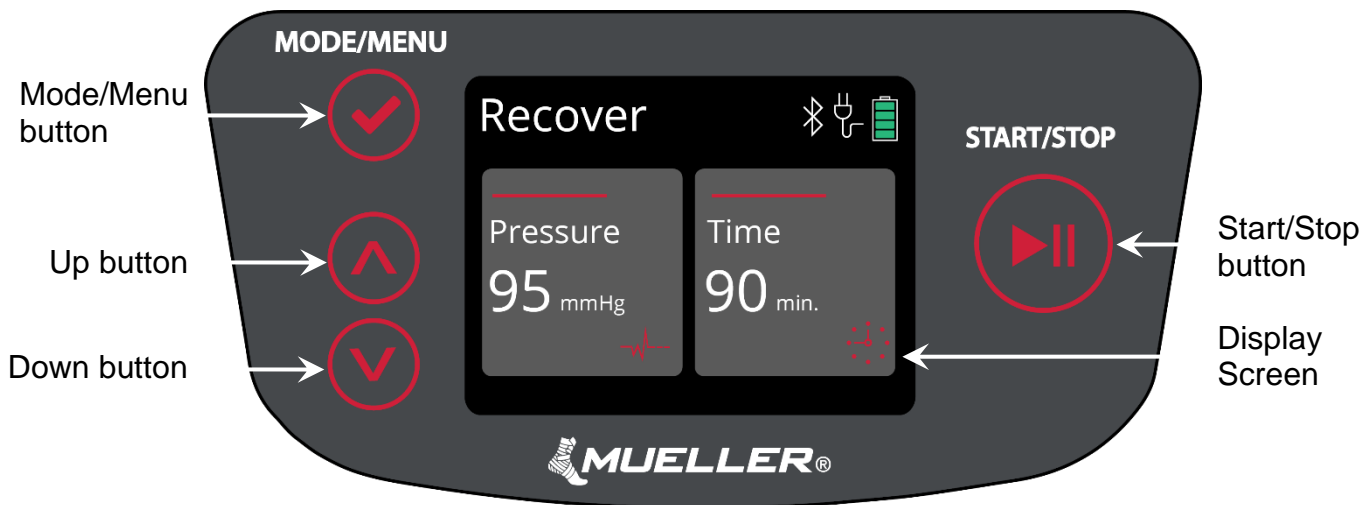
Figure 14 - The Console Operating Panel
