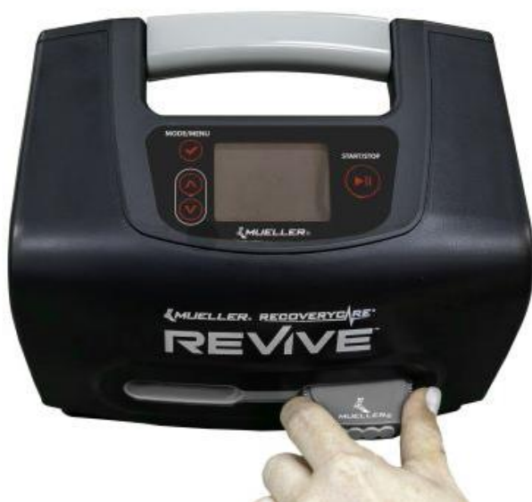
Figure 21 - Inserting the Prong Plug to Block the Unused Air Outlet for Single Garment Use
